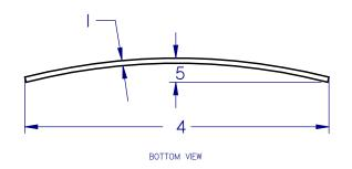
OVERALL THICKNESS MUST INCLUDE ALL INTERLAYERS, AIRSPACE, ETC.
